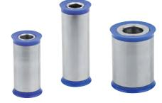
The Hygienic DESIGN spacer sleeve was specially developed for use in food-processing facilities. Special emphasis has been placed on the cleaning-optimised geometry and a surface finish of Ra  $\leq 0.8~\mu m$ . The sealing washer made from foodstuff conform plastic is exchangable.
