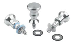
Indexing plungers are used where it is necessary to prevent changes of position due to lateral forces. A new locking position can be set only after the plunger has been manually retracted. Form C (with lockout slot) is recommended for applications where the indexing pin should remain disengaged for an extended period and be prevented from springing back.
