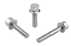
A cavity-free seal can only be assured in combination with the Hygienic USIT® seal and shim washer. The polished screws have a surface finish of Ra < 0.8  $\mu$ m. Internal transition areas with a minimum radius of 3 mm are also provided, preventing dirt particles from adhering to the components and ensuring easy cleaning.
