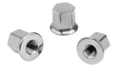
A cavity-free seal can only be assured in combination with the Hygienic USIT® seal and shim washer. The polished cap nuts have a surface finish of Ra < 0.8  $\mu$ m. Internal transition areas with a minimum radius of 3 mm are also provided, preventing dirt particles from adhering to the components and ensuring easy cleaning.
